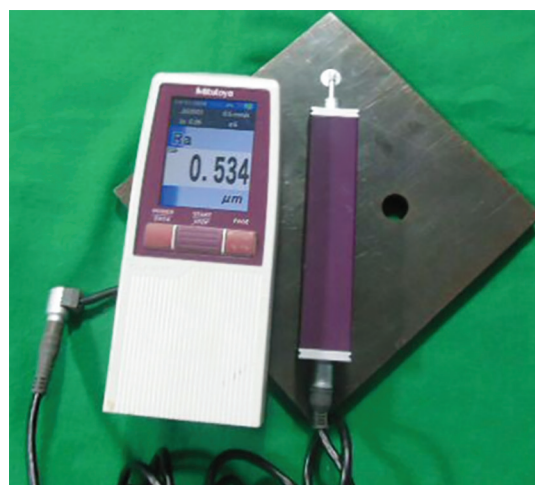
Fig. 15: Profilometer (model SJ 210 Mitutoyo, Japan)
