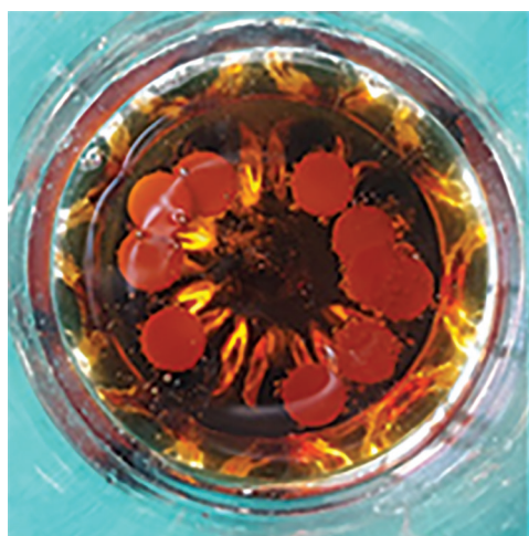
Fig. 14: Disk specimens immersed in carbonated beverage
