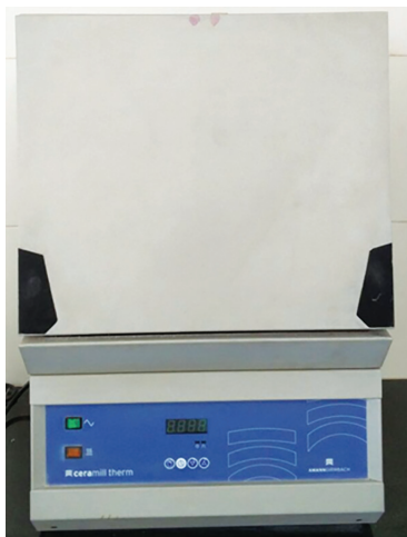
Fig. 8: Sintering furnace (Ceramill Therm furnace, Germany)
