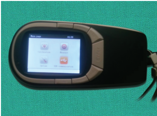
Fig. 16: Measurement of color values by reflectance spectrophotometer
